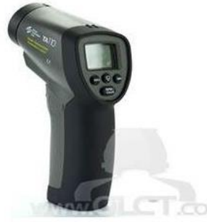
Fig. (4) A photograph of digital laser tachometer. Operating range of (1-10000) rpm, and an accuracy of \pm 0.5 rpm (Model: GTC-TA110 laser tachometer)
