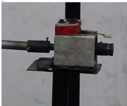
Fig. (5) A photograph of the torque meter. Operating range of (-5 to + 5) N.m, (Model: MCRT-48200v Compact digital torque meter and an accuracy of \pm 0.15 Nm)
