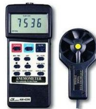
Fig. (3) A photograph of air anemometer. Operating range of (0.4 – 25.0) m/s, and an accuracy of \pm 0.2 m/s (Model: AM-4206 Anemometer)
