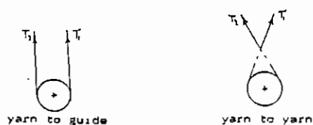
Figure(2) Principle of friction measurement
