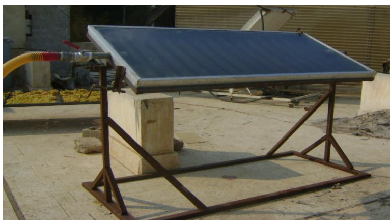
Fig. (1): Solar air heater used as an assisted system for solar dryer
