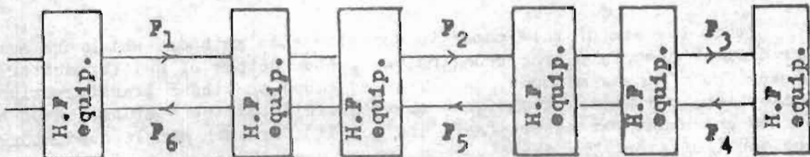
(c) duplex line operation with frequency change.
