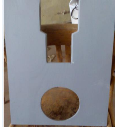
Photo 1 Combined weir with below circular gate model
