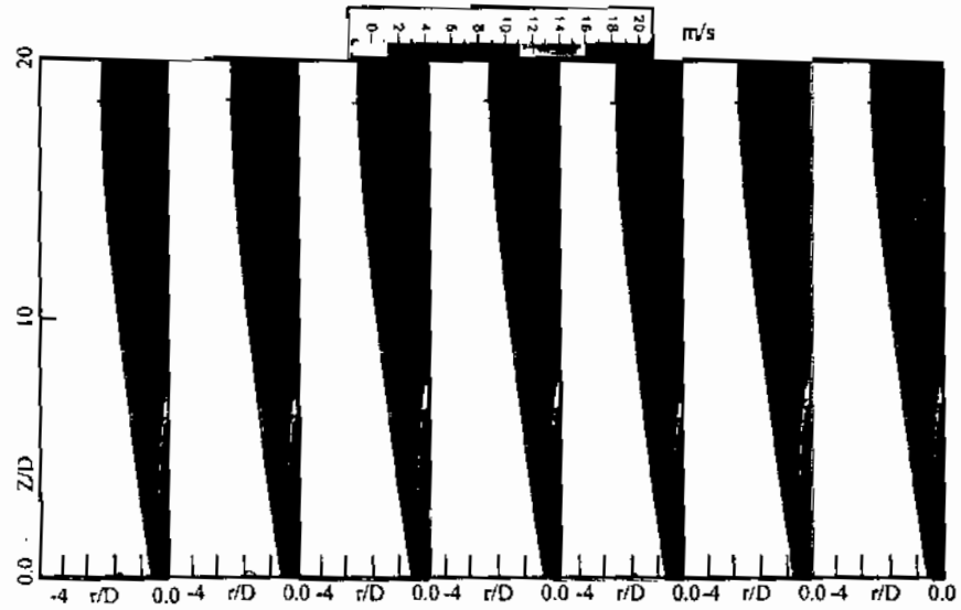
a) Baseline jet b) SJ, \alpha=0 , mr=0.055 c) SJ, \alpha=45 , mr=0.055 d) SJ, \alpha=90 , mr=0.055 e) SJ, \alpha=0 , mr=0.078 f) SJ, \alpha=45 , mr=0.078 g) SJ, \alpha=90 , mr=0.078
