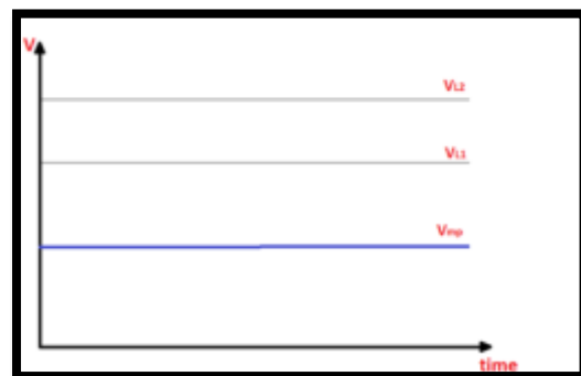
Fig. 8 Time levels of load voltage at different loads and at maximum power V_{mp}
