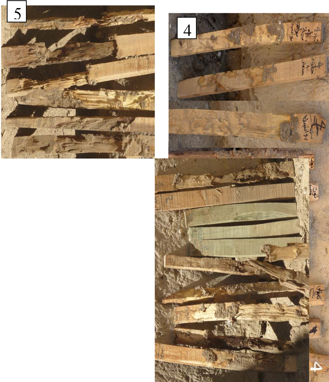
Plate (4): No injury in wood species treated with CCA compared to the other treatments (pyreban & kerosene) and untreated after one year of exposure to termites attack.
