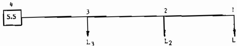
Fig.2 Single-line diagram of the test system
