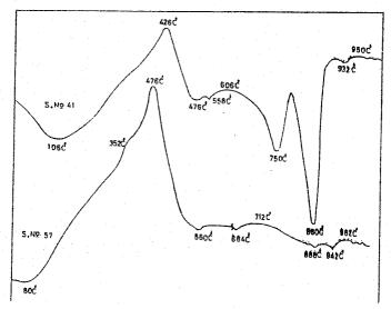
Fig. (8): Differential thermal analysis curves of some Aptian shale in Burg El-Kharita-1 well.
