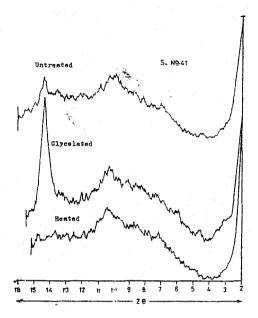
Fig. (2): Iracing of X-ray diffractometer recordings of clay size fraction of some Aptian shale in Burg El-Arab-1 well.
