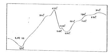
Fig. (10): Differential thermal analysis curves of Aptian shale in Alam El-Buib-1 well.
