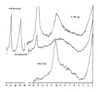
Fig. (3): Iracing of X-ray diffractometer recordings of clay size fraction of some Aptian shale in Alam El-Buib-1 well.
