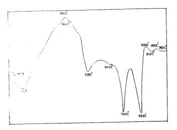
(11): Differential thermal analysis curves of Aptian shale in Qattara Rim-1 well.
