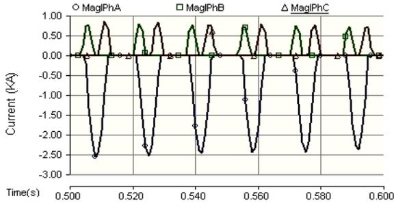
Fig. 2 Magnetizing Inrush current without residual flux
