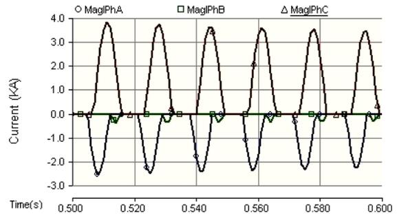
Fig. 10 Magnetizing inrush current with residual flux pattern
