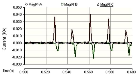
Fig. 18 Reduction of Inrush with residual flux by rapid closing strategy
