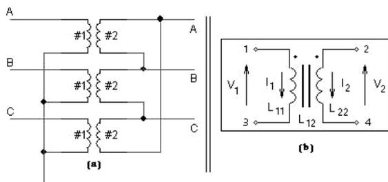
Fig. 1 PSCAD/EMTDC model (a) 3-phase, 2-winding transformer (b) classical modeling approach
