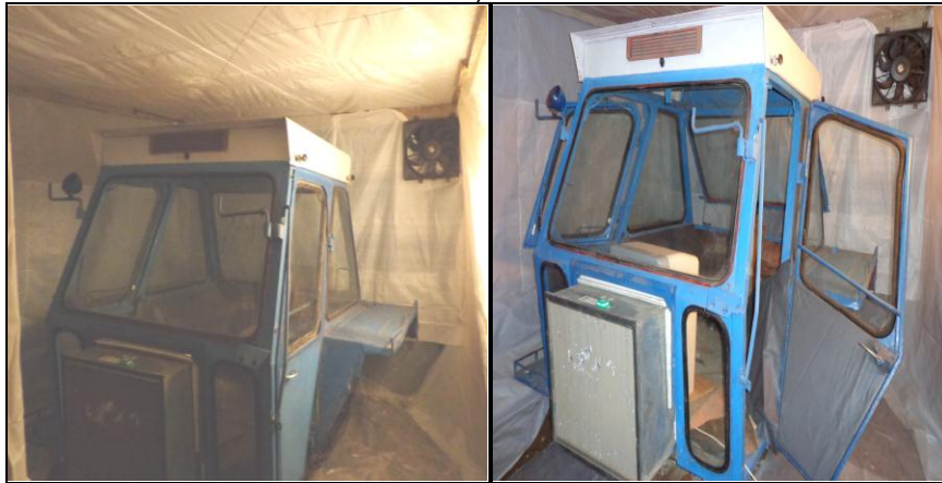
Fig. 3: The photograph of the used cab placed in a testing enclosure.
