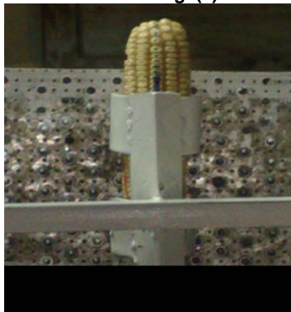
Fig. (2): The shelling plate and the holding device
