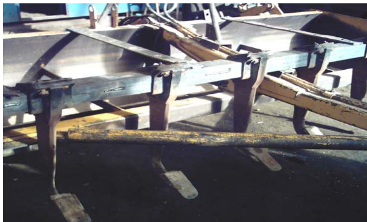
Fig. (A): Solid chisel shanks mounted of the scraper
