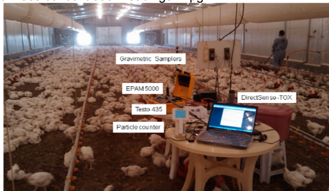
Fig. (3): Instruments used to characterize aerosol particles inside the poultry house.
