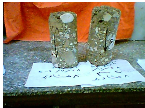
Fig. 14: Samples of the cores extracted from the trial slabs
