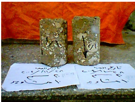
Fig. 14: Samples of the cores extracted from the trial slabs
