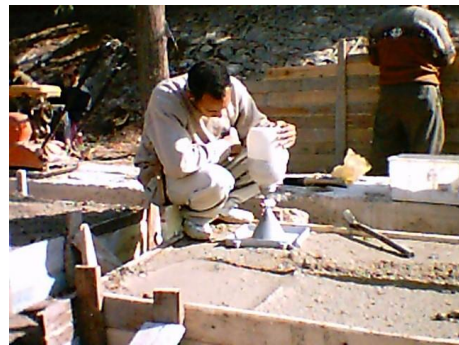
Fig. 11: Conducting sand cone test for measuring compaction efficiency
