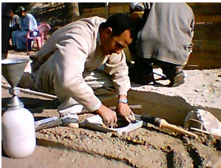
Fig. 11: Conducting sand cone test for measuring compaction efficiency
