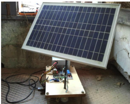
Fig. 6. Photo of Experimental Setup for smart tracker
