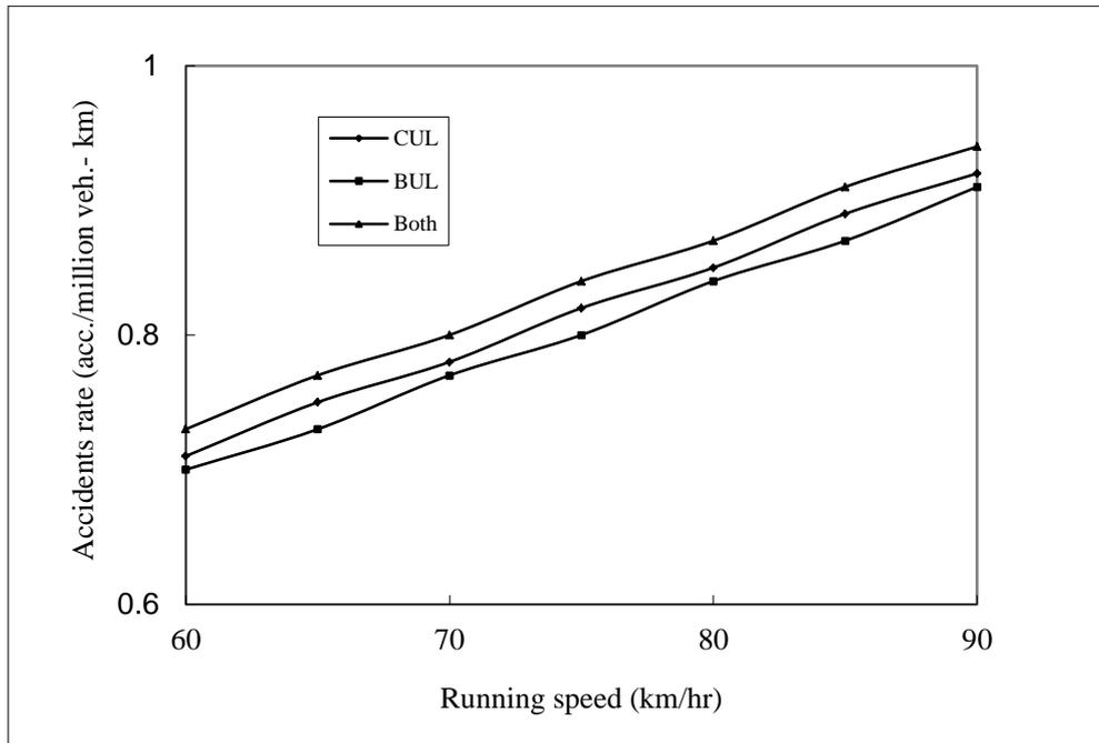
Figure (5): Relationship between Running Speed and Accidents Rate for Undivided Highways
