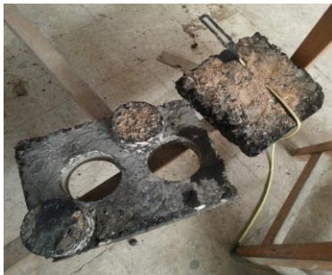
Figure 10. Cores Taken From the AC Layer After Test
