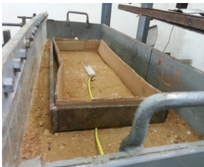
Figure 11. Strain Gages Under AC Layer
