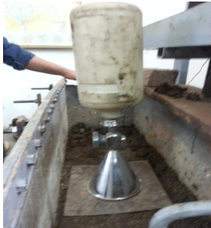
Figure 9. Sand Cone on the Sugrade Layer
