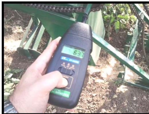
Fig (3): The Tachometer device used to determine drum Rotor speed (r.p.m) while working
