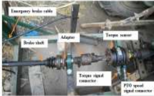
Figure 3. Torque sensor attached to tractor PTO and brake shaft
