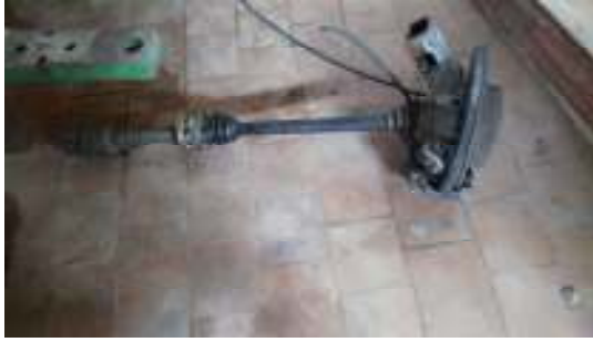
Figure 2. Brake shaft jointed to an adapter to engage with tractor PTO shaft
