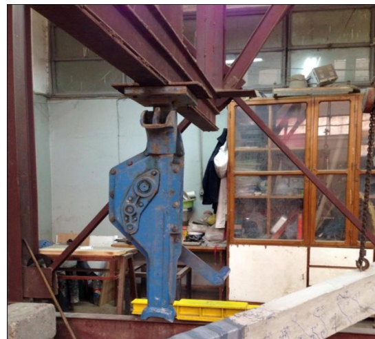
(b) Mechanical screw jack.
