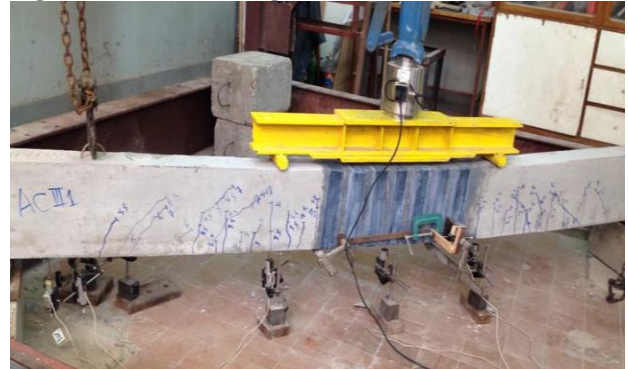
Fig.24 shows the failure mode flexure (ACIII1).
