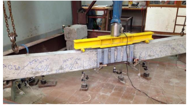
Fig.23 shows debonding in fiber (AGI4).
