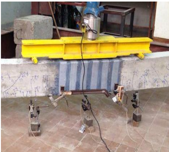
(a) Steel spreader beam and electrical load cell.
