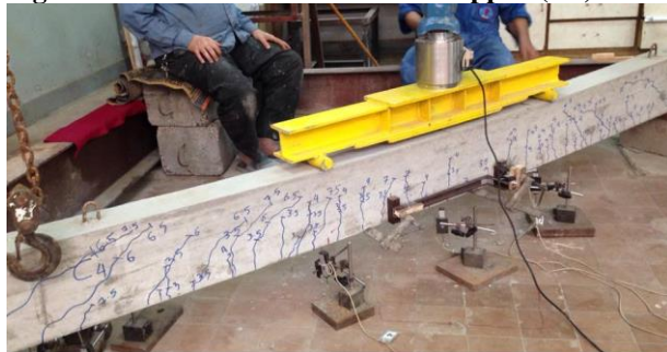
Fig.22 shows failure mode of splitting failure (A4).
