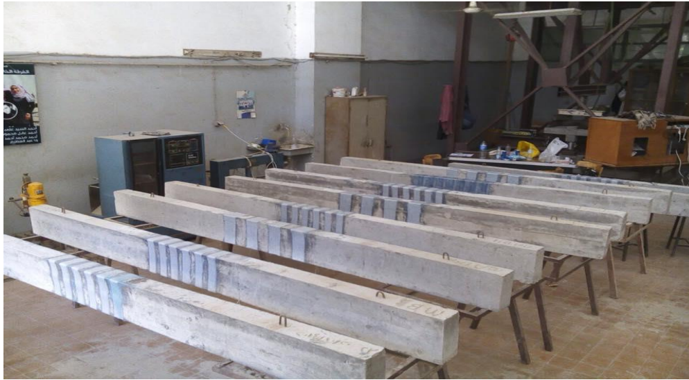
Fig. 2: Beams after strengthening.
